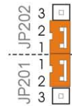
Required Jumper Placement for CN-115 Plug-in For each channel that has a CN-115 installed, pins must be jumpered as indicated above. Each channel has a jumper header next to the edge of its CN-115 header.
